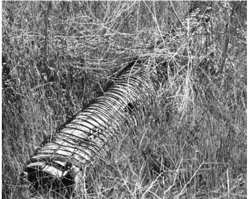
Wire wound wood pipe, abandoned in a field near Lytton.
